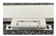
• At this point you can't see the holes to mark them so hold the hinge firmly against the frame and draw around the top and sides of the hinge with a pencil, remove the hinge and stand your frame on its side. Place the U-shaped section of the hinge within the lines you have drawn (you will notice it sits about 1mm from the front face of the screen) and mark the holes for drilling. Remove again and drill with the 2.5mm bit. See images below.
